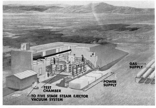
ARTIST'S DRAWING shows cutaway view of new HEAT facility planned for Sandia Laboratory. It will create the temperatures and velocities of a re-entry environment. The HEAT facility will be located in Area III adjacent to the Radiant Heat facility. Preliminary design work for the plasma arc test equipment is complete and the project is now moving into fabrication of the equipment. Total construction costs will be about \$2.5 million.
